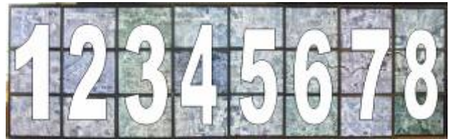
Figure 3. The display was separated into eight different columns. The total resolution of the display is 10240 X 3072 (31,457,280 pixels). The physical dimensions of the display were roughly 9 feet (2.7 m) by 3.5 feet (1 m).
